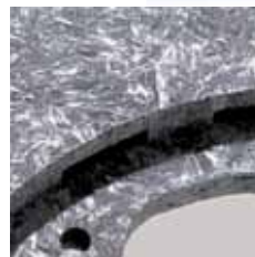
Carbon fibre-reinforced CMC material (e.g. for manufacturing high-performance brake discs in series-production vehicles)
