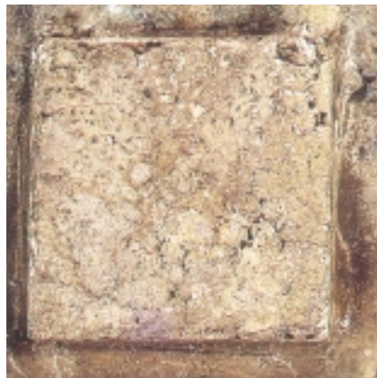
Oberfläche nach AC 4 Ag/SnO 2 SPW Surface after AC 4 Ag/SnO 2 SPW Surface après AC 4 Ag/SnO 2 SPW
