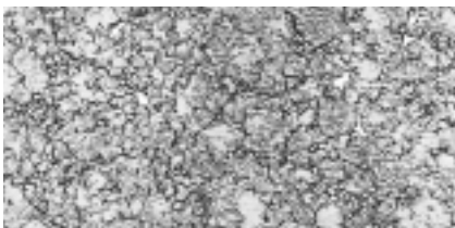
Querschliff Ag/W 20/80 Cross section Ag/W 20/80 Coupe transversale Ag/W 20/80
